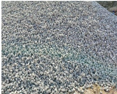
Figure 1. a) Machine crushed aggregates
