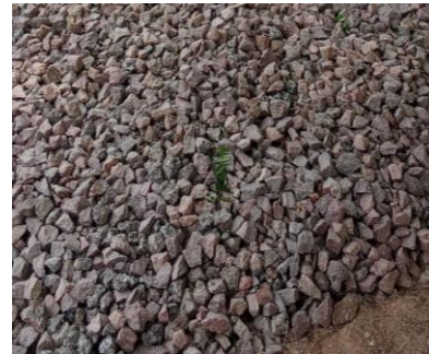
b) Hand crushed aggregates
